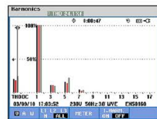
Voltage distortion THD-V of 24.1% without filtering
