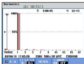
Voltage distortion THD-V of 24.1% with filtering
